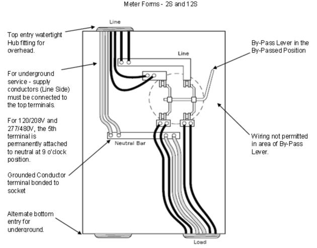
✓Applications: For Single phase 3 wire 120/240 volts or 120/208 volts or 277/480 volts 320 ampere continuous service (one meter installation).
