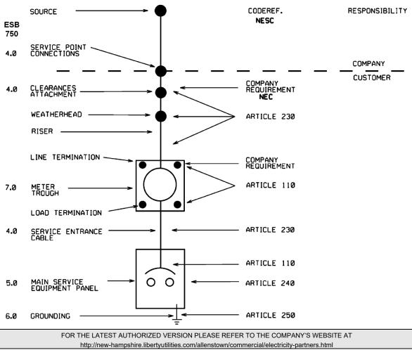
Figure 4.2.1-1 Typical Overhead Service Installation under 600V
