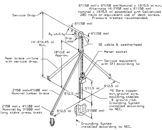
Figure 4.1.10-2 Temporary Overhead Service Below 600 volts
