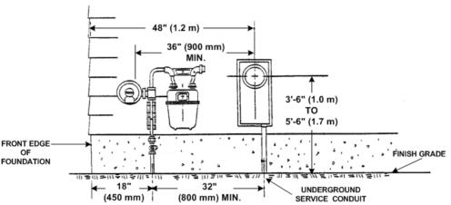
Figure 4.1.9-1 Electric Meter to Gas Meter Clearances
